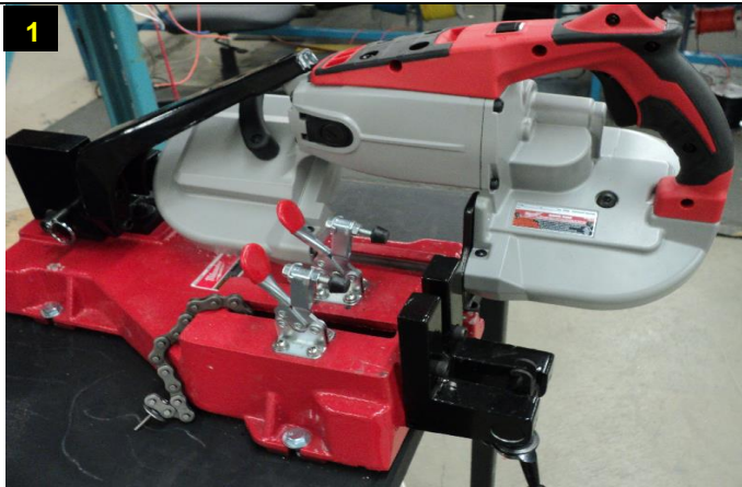
Position the band saw in the down position as shown in the picture when not in operation and pull the chain back behind the clamps.
