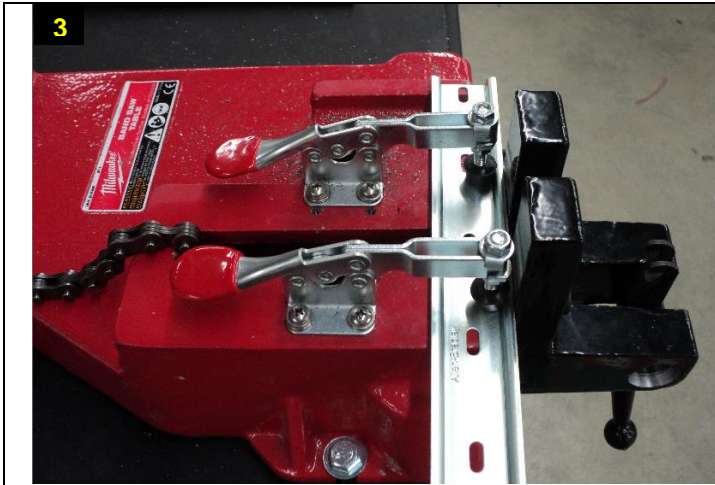
When cutting Din Rail, place the Din Rail on the work surface and against the vertical vice supports. Securely clamp the work piece in place.
