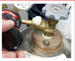
Open the tank valve (to the left) If your torch is leaking you will know right away because even if you can't hear anything, you will see bubbles develop. If you detect a leak, bring damaged equipment immediately to your supervisor.
