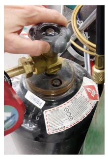
2. Adjust the Acetylene Regulator. Ensure the pressure is no more than 15psi.
