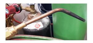
4. Check the regulators – Regulators have measurement gauges to measure the pressure of the underlying gases. Ensure that the gauges are marked clearly and are easy to read. Always remember to use acetylene under 15 psig of pressure.
