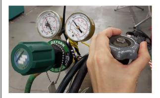
2. Adjust the working pressure no more than to 20psi.
