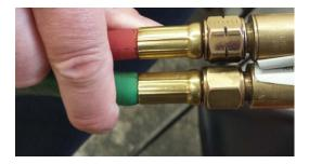
2. Open the Acetylene first by cranking the valve slightly.
