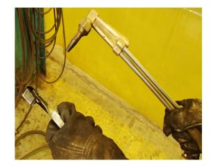
4. Adjust the Oxygen valve to the desired flame
