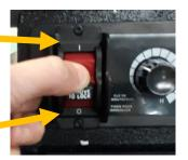
3. To lock the grinder put the switch in the "O" position, grasp the end, of the switch key, and pull it out.
