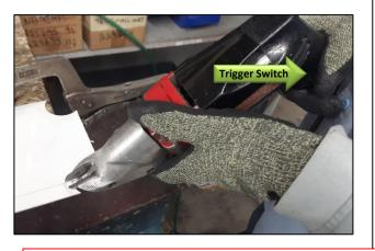
3. Hold the shear so the main body is parallel to the workpiece. Apply sufficient forward pressure to begin cutting. Too much tilt in operation will stop the cut.
