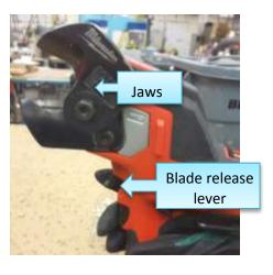
4. Press down on the trigger button and when the cut is complete, release the trigger.
