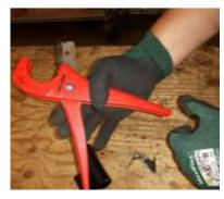
3. Mark where you want the cut to be made, then seat the pipe in the lower part of the cutter.
