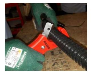
4. Squeeze the hand-grip trigger to cut the pipe. Use your other hand to hold the pipe steady as it's cut.
