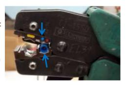
3. Twist the end of the stripped wire together. Then insert the stripped wire into the terminal lug barrel until the wire insulation butts flush against the near end of the wire barrel.
